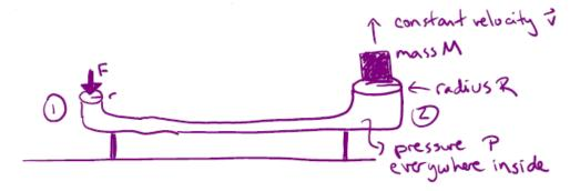
You push down on side 1 (the skinny side) with a force  $\vec{F}$  and want to raise the mass M which sits on side 2 (the fat side) at a constant slow velocity. Static fluids are able to equilibrate pressure everywhere within the fluid. Use the momentum principle to solve for the value of the force F required to lift the mass M, in terms of such variables as (M, r, R, v, q)etc.) Be sure to specify an appropriate choice of system and surroundings.
