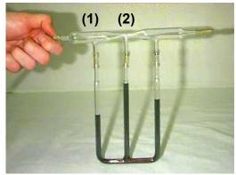
The flow meter is the fork-like set of tubes connected to the bottom. The dark fluid can flow freely within the flow meter, and is observed to have risen to the largest height within the middle
