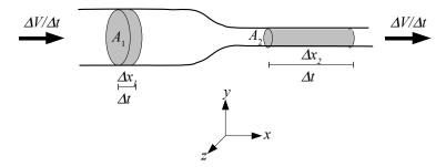
We'll assume that the fluid is incompressible (e.g. a liquid, rather than a gas), so it can't just squeeze itself down to a smaller size. As the fluid moves from left to right, it is confined to a narrower space, but the same volume of fluid/sec needs to keep moving through the pipe. Therefore, the flow rate is constant and from our definition of flow rate we know that
